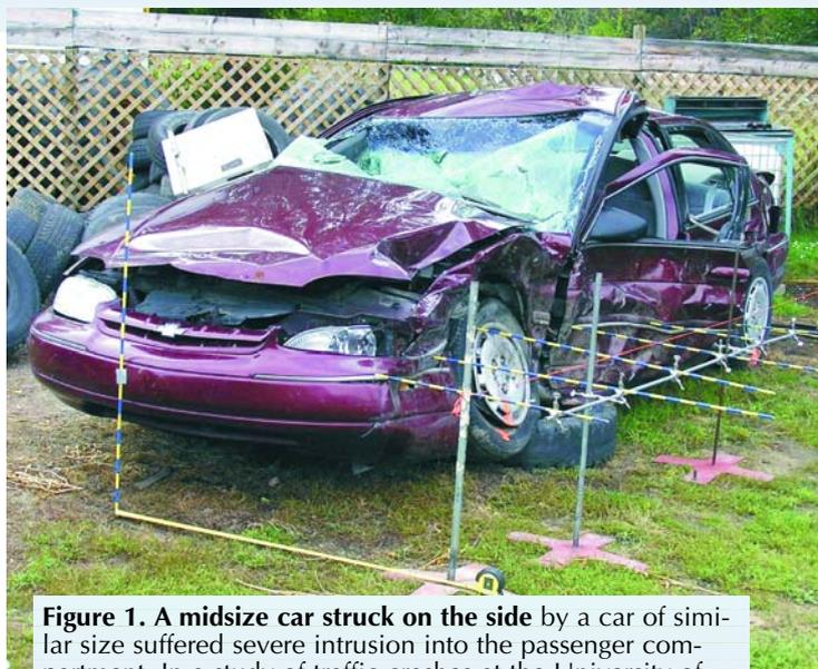
**Figure 1.** A midsize car struck on the side by a car of similar size suffered severe intrusion into the passenger compartment. In a study of traffic crashes at the University of Michigan, a measuring system determines horizontal deformations of the car relative to its original surface. As described in the article, the analysis of such actual road accidents, together with laboratory test crashes, provides guidance for safer vehicle design. (Photo courtesy of Joel MacWilliams.)
